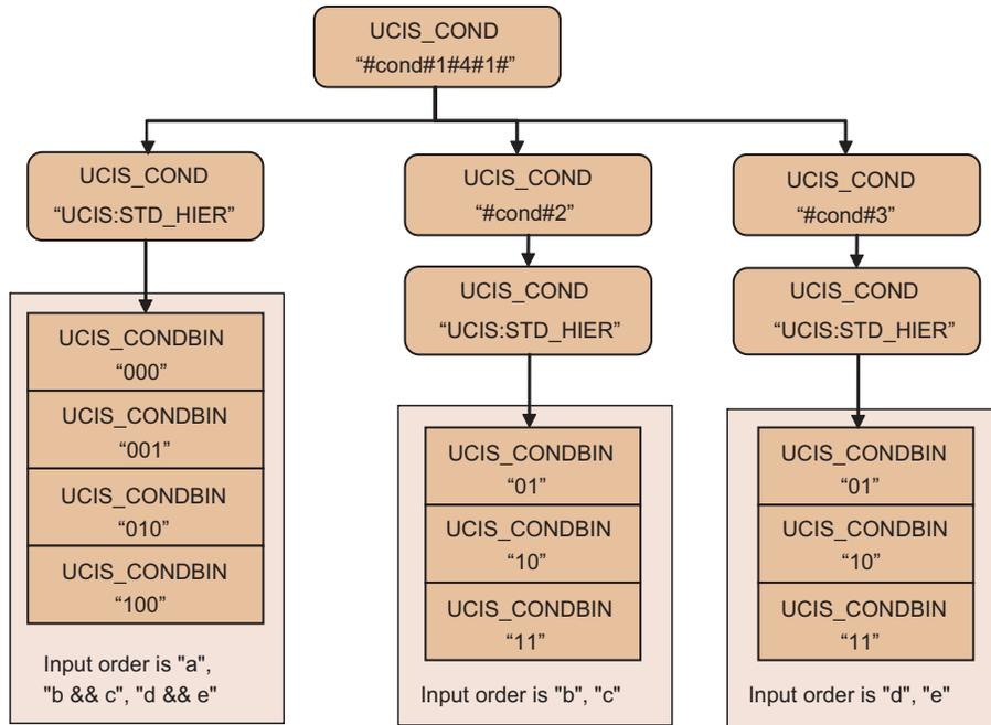
**Figure 28—Example of condition with sensitized vector bins**
