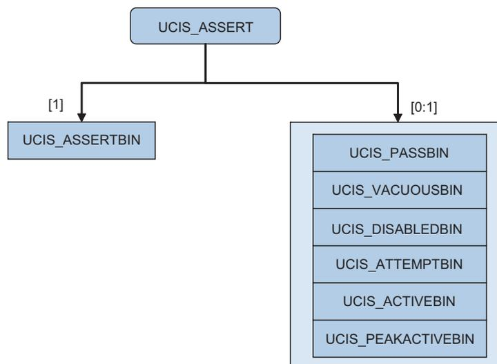
Figure 40—Assertion coverage structural model
