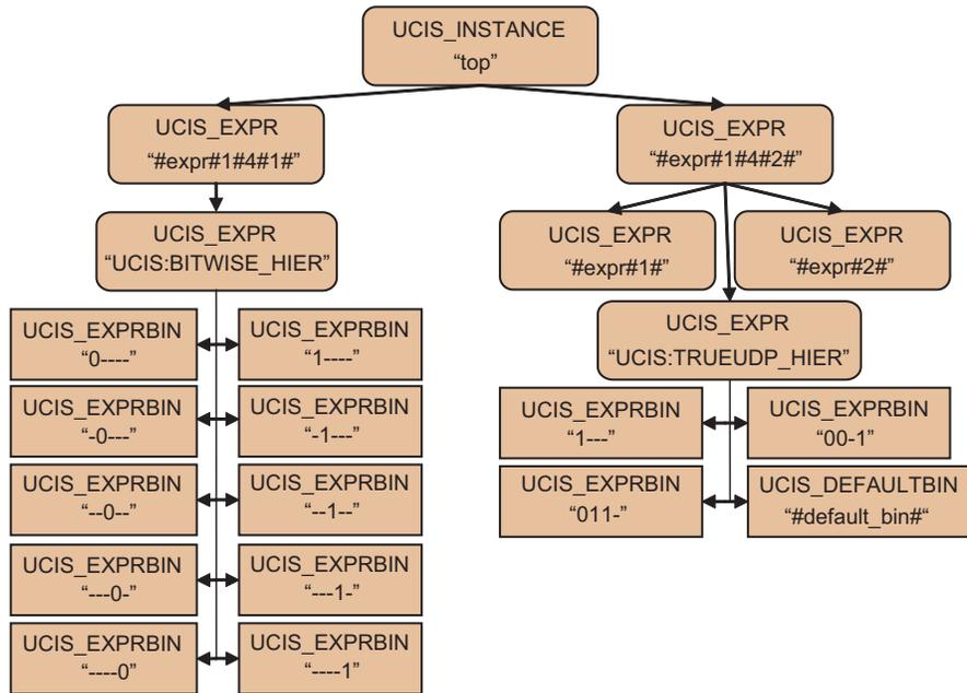
**Figure 27—Example of condition and expression hierarchical model**
