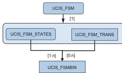
Figure 36—FSM coverage structural model
