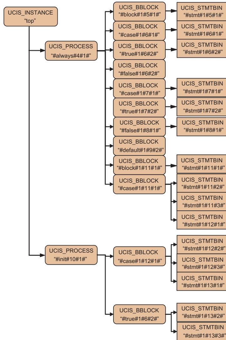
Figure 24—Example of block coverage with UCIS\_BBLOCK flattened
