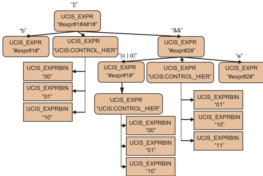
**Figure 30—UCIS\_CONTROL metric for an assignment statement**
