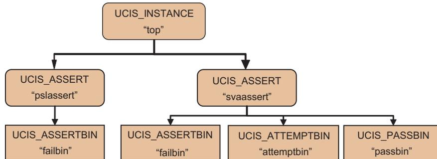
**Figure 41—Example of SVA and PSL assertion coverage**
