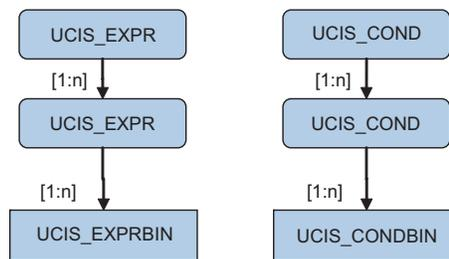
Figure 25—Example of condition and expression structural model
