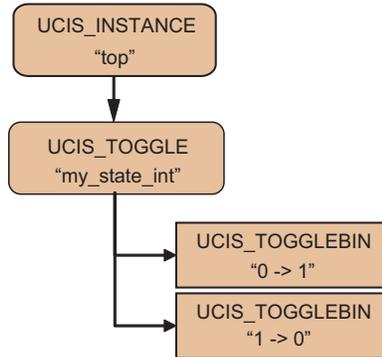
**Figure 34—UCIS:2STOGGLE without metric tye scope**
